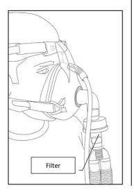
Dual limb no Bacterial-Viral filter – For integral filtering ventilators
