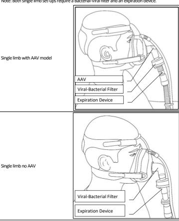
Note: The Standard elbow (Blue Elbow) model must be used, with either ventilator, with adequate alarms or a circuit that contains an AAV to provide access to room air in case of ventilator malfunction
